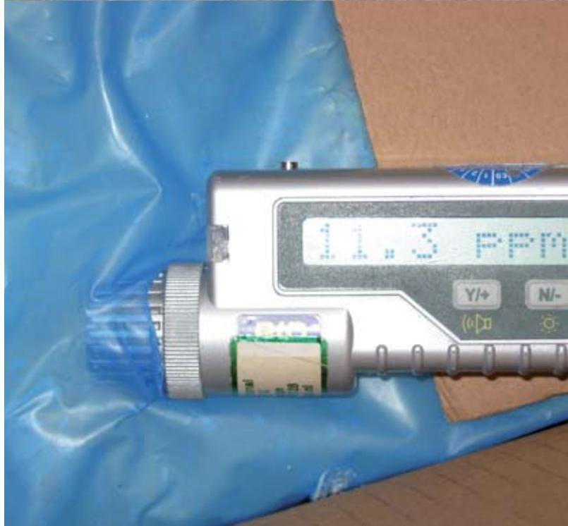
Measuring during testing for product gases in packaging.
