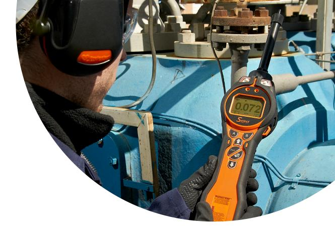
A revolutionary hand-held detector, Tiger Select can be operated either with a benzene pre-filter tube to detect benzene selectively, or without to detect total aromatic compounds (TAC). For simplicity and ease of use, the Tiger Select has been split into two, user-friendly modes: Basic and Advanced. Both modes are user-selectable.
